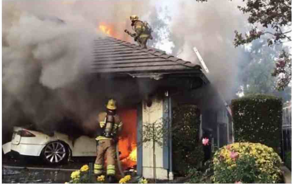
During a Tesla crash in Lake Forest, California, in 2017, the battery fire reignited three times (Credit: Orange County Fire Authority)
